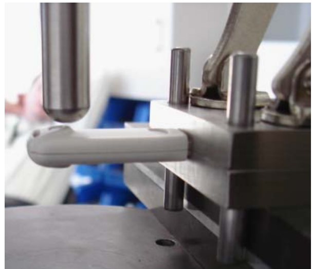
Typical setup of a USB key in the fixture with the probe positioned above the specimen
